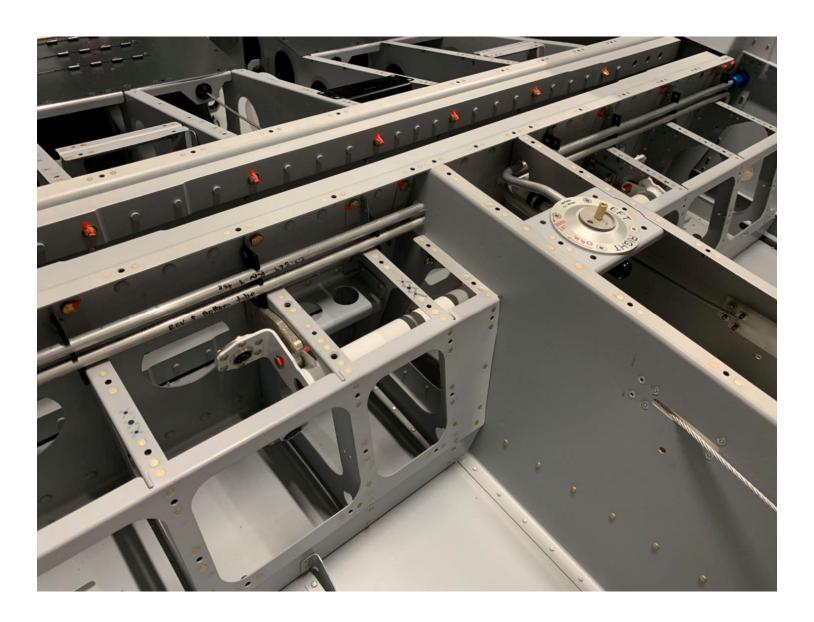
Here is a picture of the CNC Machined angles that are included with the kit for mounting your fuel pump setup. These angles were drilled for SDS pump mounts and may need modification for EFII. Mount all hoses first to ensure everything is in correct location before drilling new holes in angles. VERY IMPORTANT NOTE: You will want to trim the aft vertical edge at an angle and taper it so that you run no risk of interference with your controls at their extreme positions. See next page.
