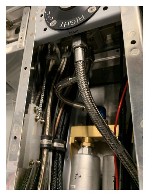
CENTER TUNNEL FLEX HOSES "ASF 140RT-7 RX H3" – Long hose to Firewall -This is the fuel RETURN LINE. It should go into the fuel return port on the Andair Valve.
