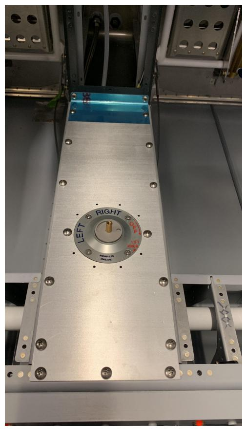
Please note in this image that you will receive two doublers. One is the ring doubler (Not seen) for the valve itself and one is a tunnel doubler plate. You will cut the Vans original tunnel cover short and utilize ours over the top of it. Cut the Vans cover so it remains as long as possible but doesn't interfere with the valve.
